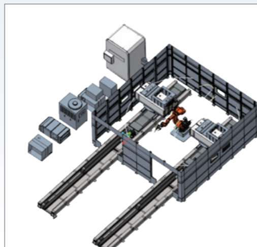
地面式机械手+移动地轨+旋转变位机 Ground manipulator + mobile ground rail + rotary positioner
