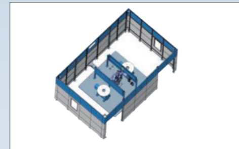
配置双工位 P 型双轴变位机 Equipped with double-station P-type double-axis positioner
