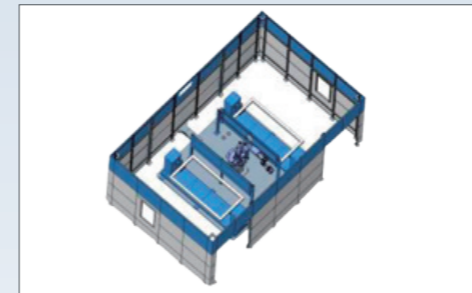
配置双工位首尾相连框架式单轴变位机 Configure double-station end-to-end frame type single-axis positioner
